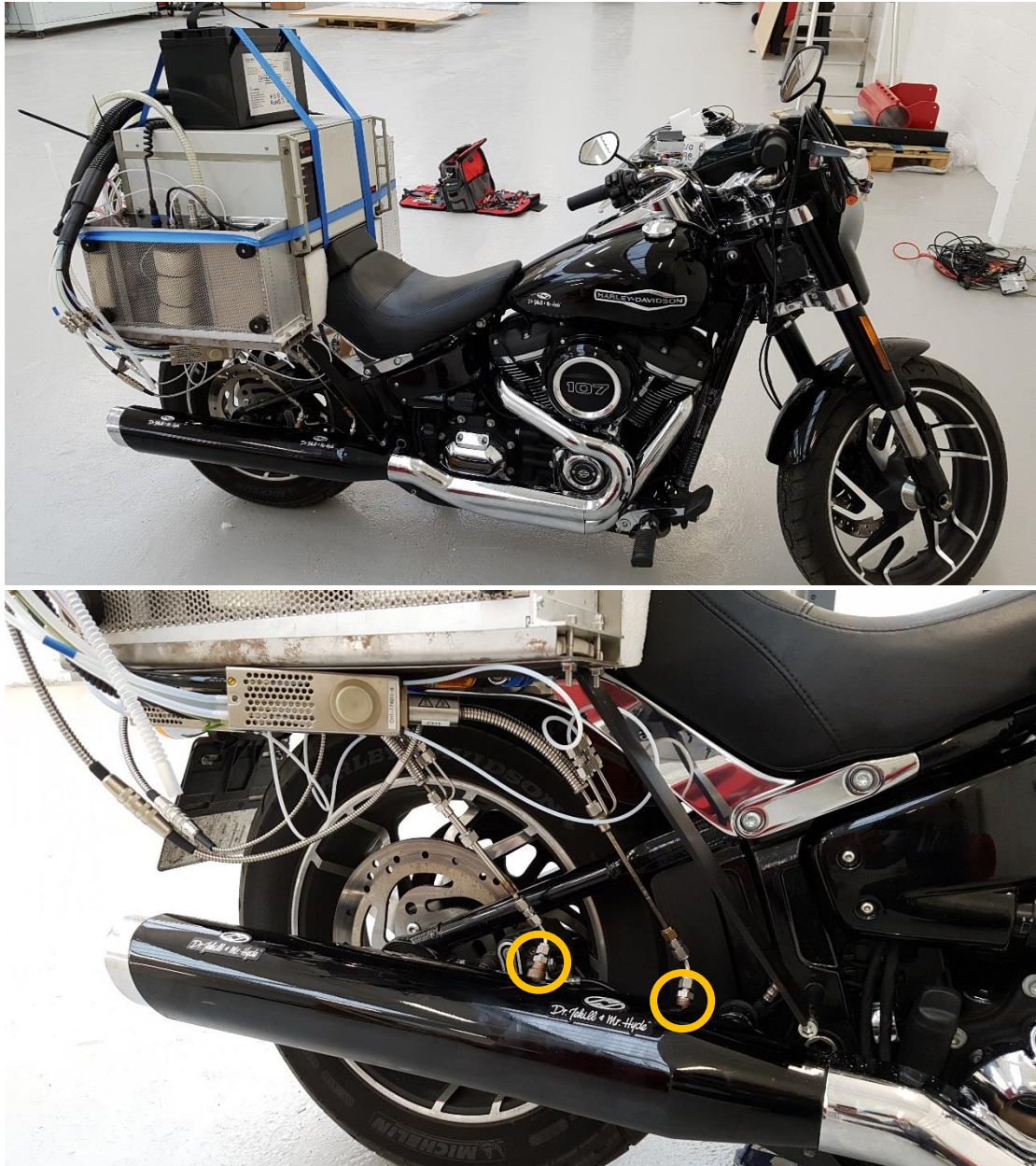
Figure 1: Two-channel fast NOx analyzer sampling engine-out and tailpipe [NO]
