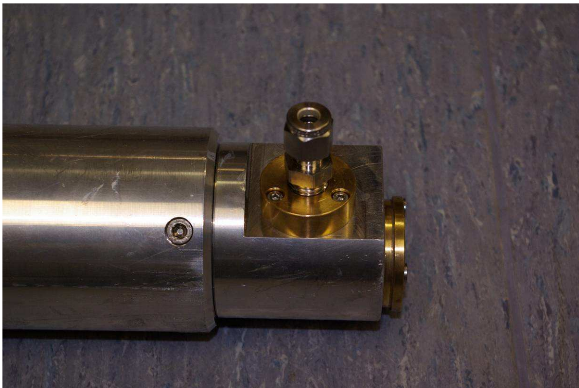
Figure 3 Heated line with SS-6M0-1-4RT Swagelok fitted
